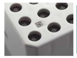
The base of each cryogenic box has a 2D barcode laser etched on to the base. This is used when scanning the tubes, as the Ziath DataPaq<sup>™</sup> 2D barcode scanning software uses this extra 2D barcode to determine the orientation of the rack on the scanner bed.
